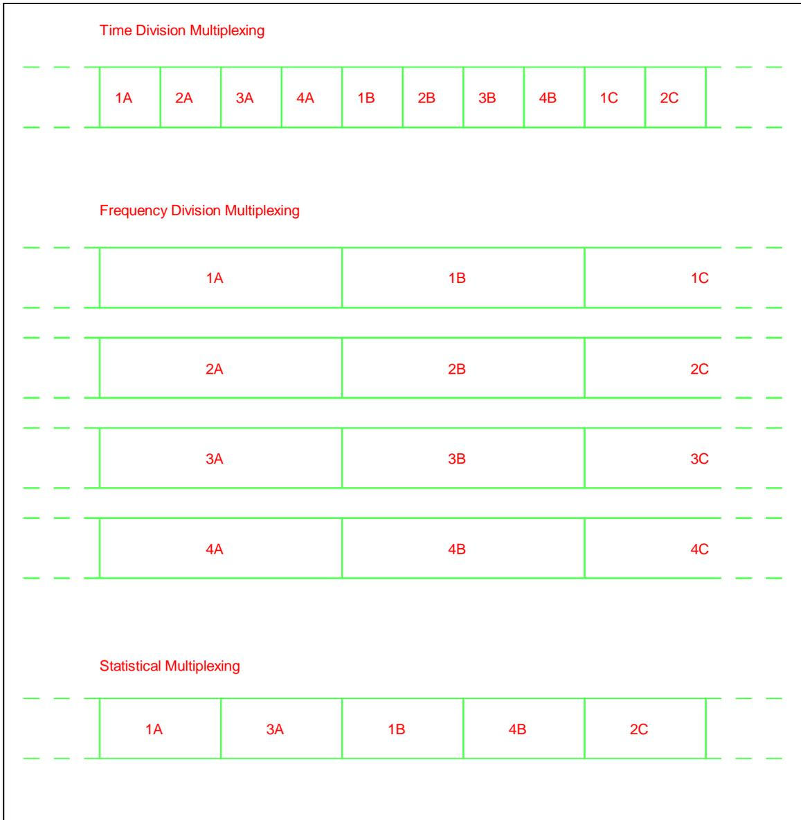
**Figure 3 Methods of multiplexing**
